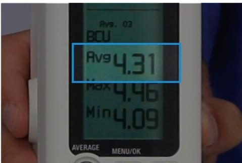
The BC-10 Plus takes as many measurements as required, and can store up to 16 readings at a time. To display the average of the stored readings, simply press the Average Button.
