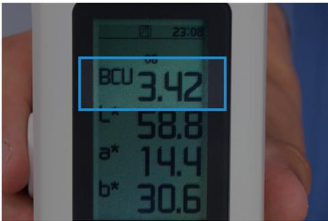
A Baking Contrast Unit is the measure of the lightness or darkness of a product. BCUs range from 0 for the darkest to 5.25 for the lightest. Each change of 0.1 BCU equals approximately one discernible shade to the human eye.
