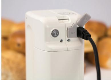
3. By connecting a printer to the BC-10 Plus, you can print out measuring data.
